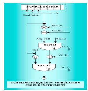
Figure 7. A graphic illustration of the csound instrument used for the homomorphic mappings experiment.
